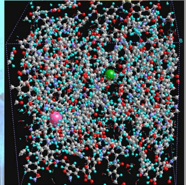
Advanced water purification and desalinization begins with a detailed understanding of how ions in water interact with purification membranes. This dynamic computer simulation shows sodium (pink) and chlorine (green) ions inside a polyamide membrane. *Shannon, 0120978.*
