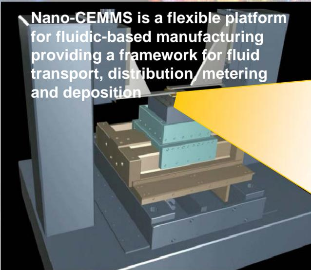
An interchangeable toolbit provides process flexibility and helps bridge scales from the macroscale to the meso and microscales.
