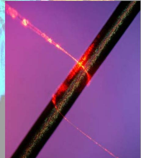
Light moves along a nanowire, pictured here wrapped around a human hair. Controlling light at the nanoscale could allow many applications, such as high-resolution sensors and optical transistors.
