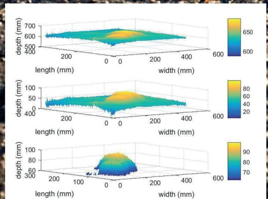
Early testing of the pothole scanner shows promising results. Above, data show that the scanner has successfully measured the size and depth of a pothole.
