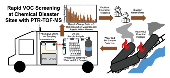
Through a newly-developed rapid screening method, spill responders will be able to more quickly and precisely test for volatile chemicals. This test can be used in a number of hazardous spill scenarios to provide responders faster results when checking for volatility in the soil, water, and air.
