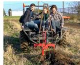
This design team exists to construct and install a high/low driveline option to provide custom gearing ratios for more flexible use. The design uses a motorcycle transmission commonly found in Africa to help provide a 3-way reduction for different speeds/torques. This allows end users to use the PUP to enact a wider range of activities, ranging from high torque applications (plowing) to high speed applications like travel.
