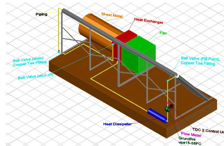
Figure 1: The fourth version of our design produced in AutoCAD.
