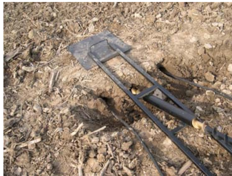
This apparatus is used for drilling holes beneath the soil surface. A large cordless drill makes the process almost effortless.
