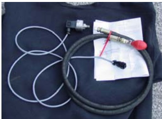
Pressure Sensing Bulb, Hose, and Pressure Transducer
