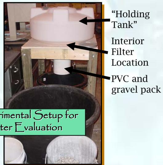
Experimental Setup for Filter Evaluation
