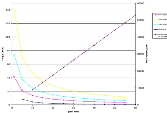
The graph shows the torque and motor speed required for our vehicle to travel 10 mph on different road slopes.
